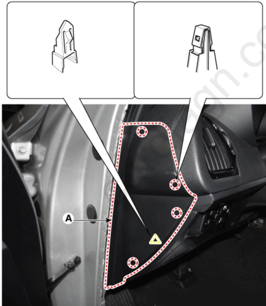
2. Separate the crash pad lower panel (A) after loosening the bolts and screws.
