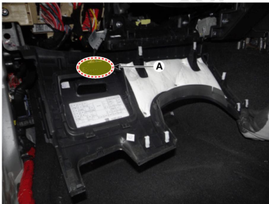
4. Remove the crash pad garnish [LH] (A) after loosening the mounting screws.
