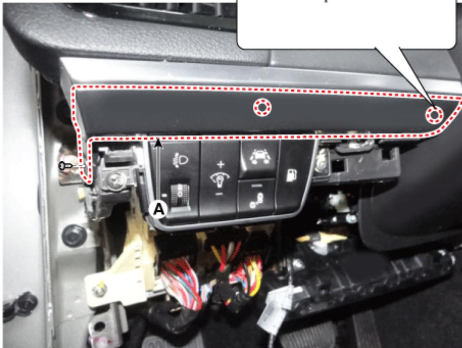
5. Remove the crash pad driver side panel (A) after loosening the mounting screws.
