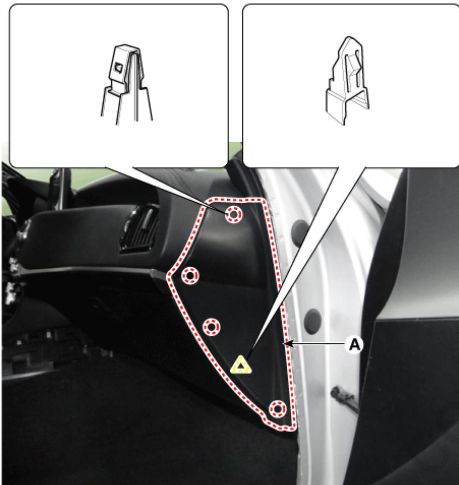
7. Remove the crash pad garnish [RH] (A) after loosening the mounting screws.
